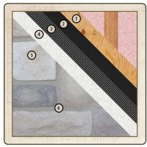
Rigid backwall (sheathing, in this example), 2 weather-resistant barrier, 3 metal lath, 4 mortar setting bed, 5 manufactured stone, 6 mortar joint.
